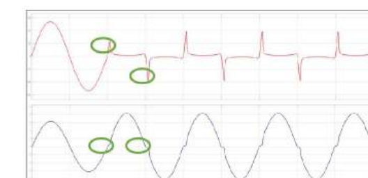
Current and voltage waves of pure resistive arc discharge
