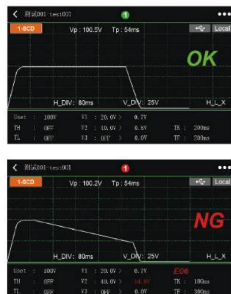
Figure 1/2 Test process of qualified and unqualified 5uF battery cell under 100V voltage (voltage rise time 54ms)
